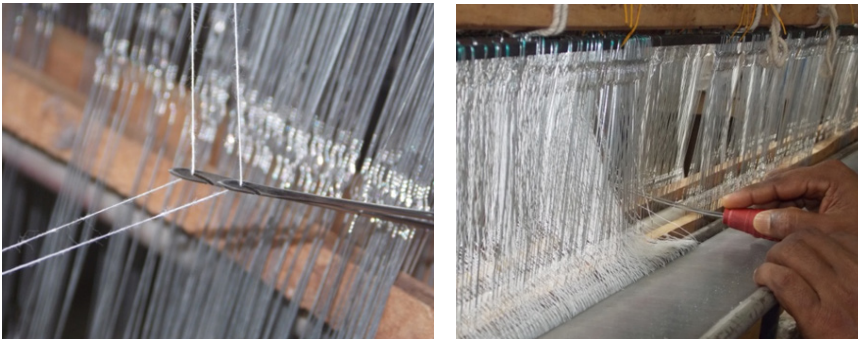
Figure 8: Denting in & drawing operation.
