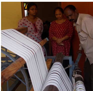
Figure 10: Tying the threads to the warp beam.
