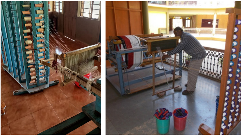
Figure 7: bobbins arranged on a creel
