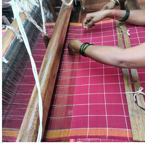
Figure 11: weaving on the loom. (sari without the dobby border)
