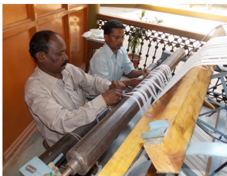
Figure 10: Tying the threads to the warp beam.
